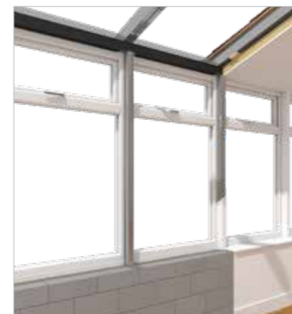
Structural Support mullions capable of holding the full weight of the tiled roof system, where frames are not adequately reinforced
